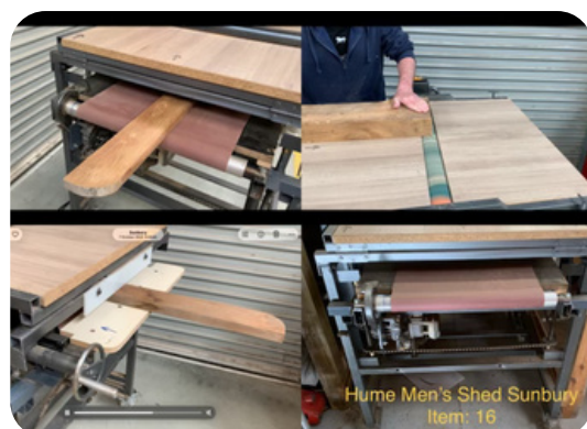
SHOP BUILT DRUM SANDER 240V 600MM WIDE TOP, 400MM WIDE POWER FED
