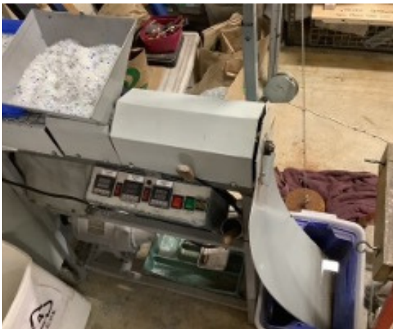
8. The Shed made plastic extruding machine – the extrusion machine in action
