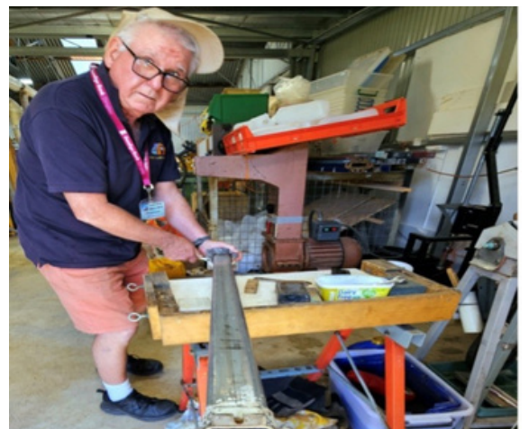
6. Damien resetting a die – showing the die setup process
