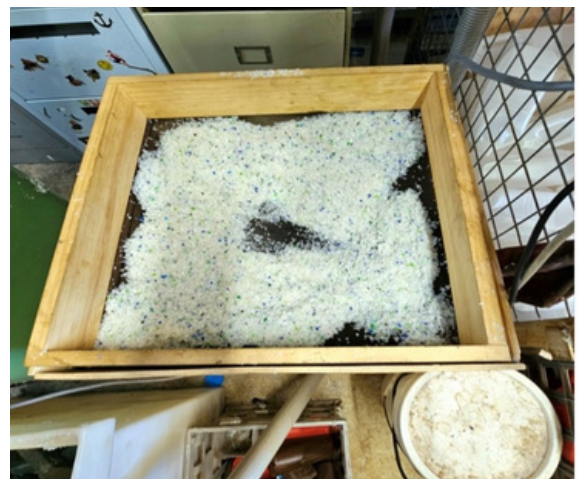
3. Plastic granules are sieved for the correct size – granules are sorted to the right size for extrusion
