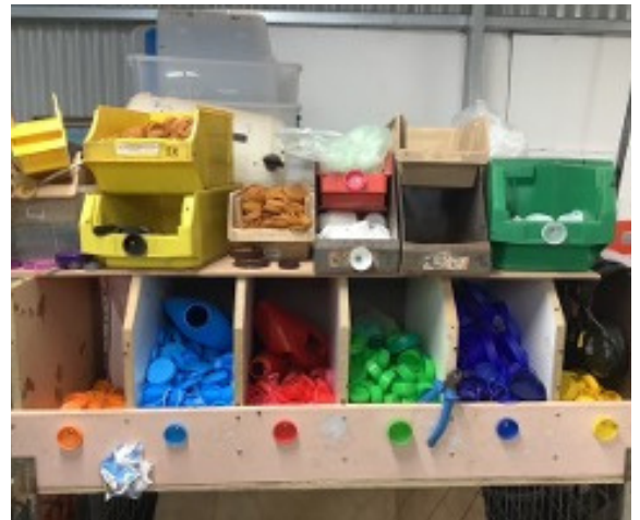
4. Plastic caps are used to provide colour – colour is added to the mix
