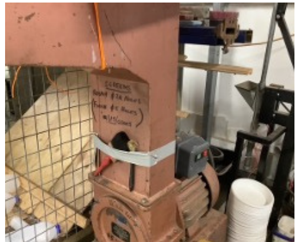
2. The very noisy chopper/ granulator – the plastic is chopped and granulated
