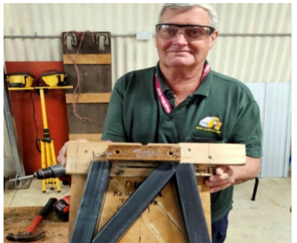
11. Kevin with wooden jig for assembling the legs of bench seat – assembly in progress
