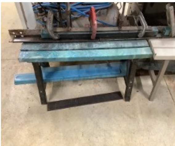
9. Extrusions are still pliable and have to be clamped to keep straight – the freshly extruded plastic being shaped
