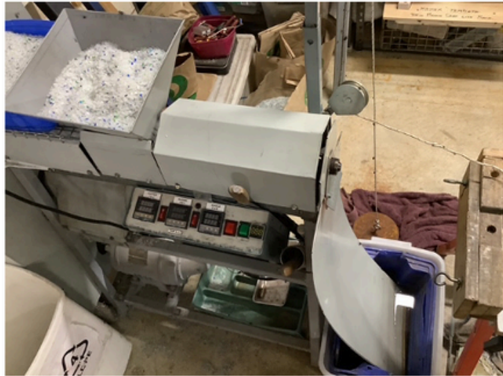
The heart of the recycling process is the extrusion machine & mould which shapes the heated recycled plastic
